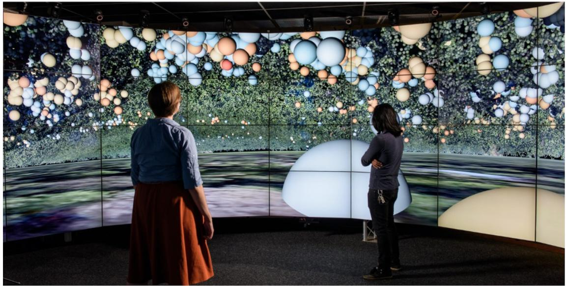
A data visualization of a glass fissure molecular dynamics nanoscale simulation computed at Argonne National Laboratory's Leadership Computing Facility can be streamed to COMPaaS DLV over a high-performance network and simultaneously displayed with additional information on EVL's CAVE2™ hybrid reality display. (Photo courtesy of Lance Long, EVL)
