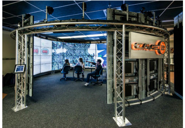
A data visualization of a glass fissure molecular dynamics nanoscale simulation computed at Argonne National Laboratory's Leadership Computing Facility can be streamed to COMPaaS DLV over a high-performance network and simultaneously displayed with additional information on EVL's CAVE2™ hybrid reality display. (Photo courtesy of Lance Long, EVL)
