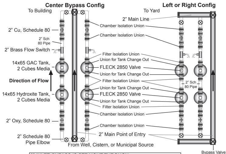
2" INLET, BYPASS IS STRAIGHT THROUGH
