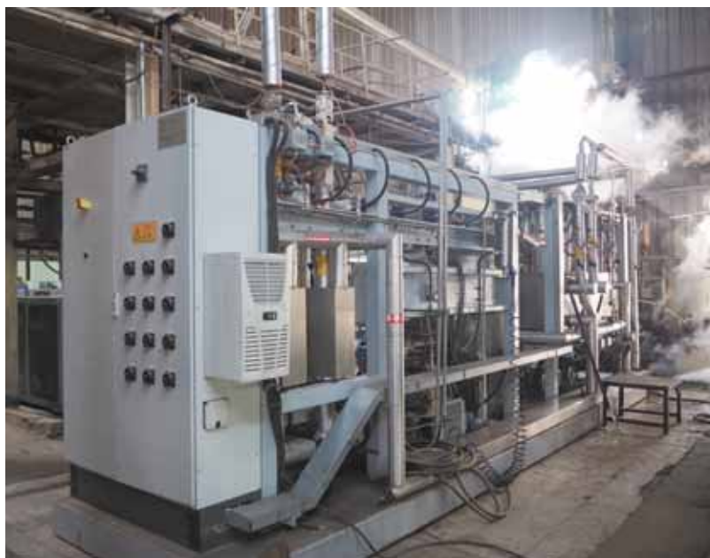
Within a few hours, SMARTTECH's wax suspension system can be installed between the existing wax system and the refiner in the plant. It does not require any additional labour to operate.
