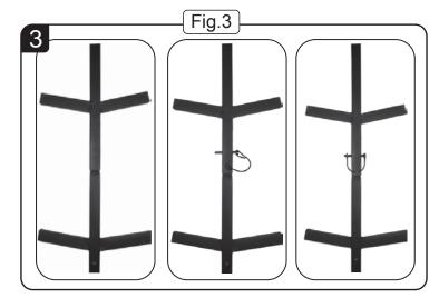
Insert the rest of the sections together by following the above steps. Make sure all connections are tightened securely. Insert one quickclip through each section at each insertion point. (See Fig. 3)
