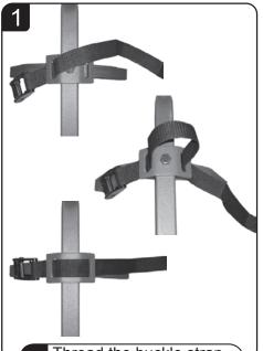
Thread the buckle strap through one end of the bracket, over the top of the bracket. Then through the other side of the bracket. Pull the strap all the way through so the buckle end is against the bracket. The straps will be attached to the bracket and hang freely until the Stick Ladder is ready to be secured to the tree.
