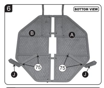
With the platform still upside down. Attach Rear Leg Braces to the rear of the platform using **2-M8x75mm PURPLE Bolts** for each Rear Leg Brace.
