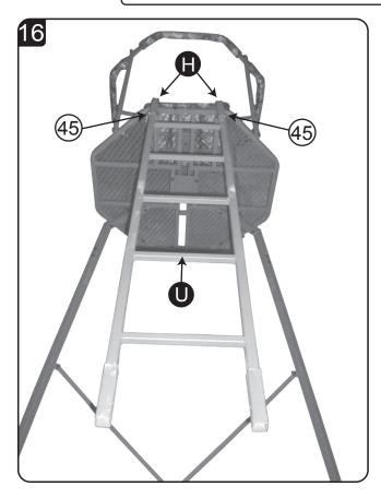
Insert Top Ladder Section (1) into Handle Rails (1). The brackets on the Ladder Section MUST be facing towards the inside of the stand. Secure using 1-M8x45mm YELLOW Bolt (45) on each side.
