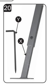
Insert Anchor Pin or through the hole on each Foot X when the stand is in desired position.
