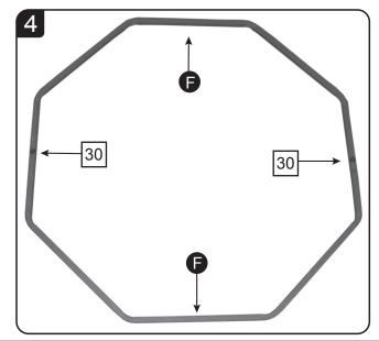
Slide both halves of Shooting Rail together and secure with 1-M6x30mm WHITE Bolt 30 on each side. Set aside for future use.
