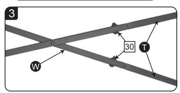
Insert the crimped end of Male Brace into the end of Cross Brace near the pivot point. Insert 1-M6x30mm WHITE Bolt 100 at each point. Do this for ALL remaining Cross Braces. Set aside for future use.
