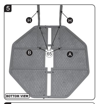
Turn the assembled platform over so that the top of the platform is on the ground.
