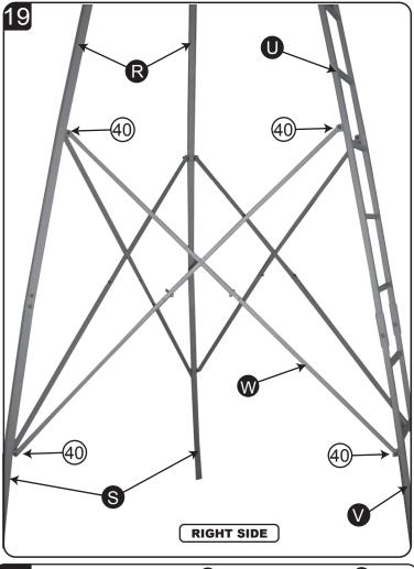
Attach another Cross Brace **(W)** to Top Ladder Section **(U)** and Lower Leg **(S)**. Attach the same Cross Brace to Bottom Ladder Section **(V)** and Upper Leg **(R)** using 1-M8x40mm BLUE Bolt **(40)** at each point. Attach Braces to the OUTSIDE of the Brackets.
