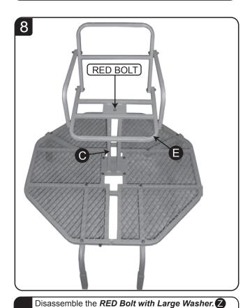
Place the Large Washer on top of the Seat Pedestal . Hold the assembled Seat on the Seat Pedestal. Place a metal washer onto the *RED* bolt, then insert a nylon washer on the bolt. Insert the bolt through the Seat Platform, Large Washer, and the Seat Pedestal. Place another nylon washer onto the bolt, then the last metal washer and tighten the nut.
