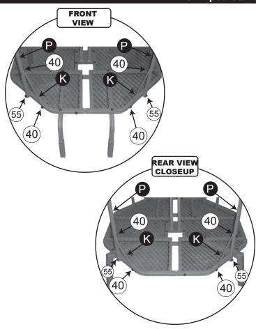
Attach Shooting Rail Support P the assembled platform using 1-M8x55mm BLACK Bolt 55 for each piece. (The two holes on the Shooting Rail Support will be on the bottom. See Close-Up Photos for correct placement).
