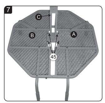
Turn the platform upright. Attach Seat Pedestal to the center of the platform using 4-M8x45mm YELLOW Bolts. (45)
