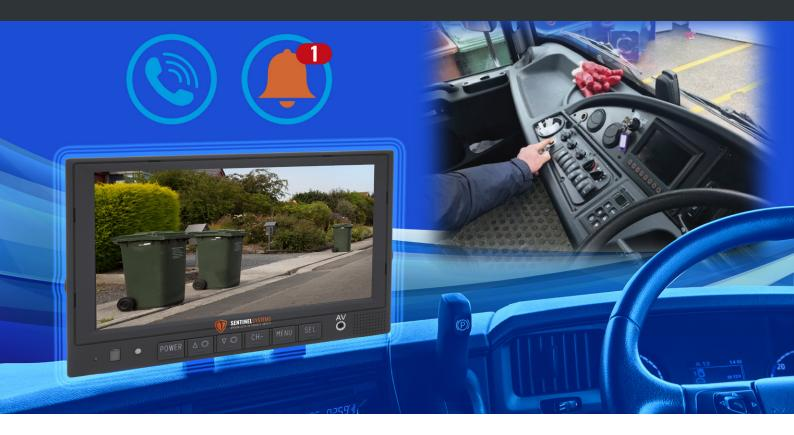
Make trawling through days of footage a thing of the past with the Sentinel Incident Button. Utilising our top of the range DVR's abilities, combined with our premium software suite, the driver is able to highlight moments of interest at the push of a button.
