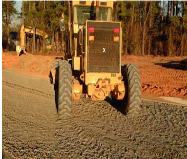
Photo 2. This photo illustrates the rear of the grader used at the time of the incident. The backup alarm is positioned behind the grill work and is marked with an X.
