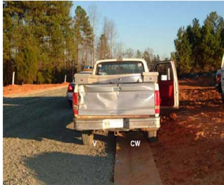
Photo 1: This photo illustrates the approximate location of the victim (V) and the coworker (CW) at the time of the incident. The tailgate of the truck shows damage that resulted when the grader struck the truck.
