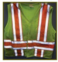
Characteristics: Good reflectivity but has some soiling and light fading of material. \*Note: This picture was taken with a flash and simulates nighttime conditions.
