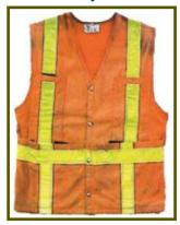
Characteristics: little or no reflectivity, and soiled and faded material.
