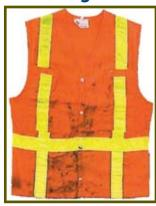
Characteristics: Good reflectivity although the vest has some soiling and light fading.
