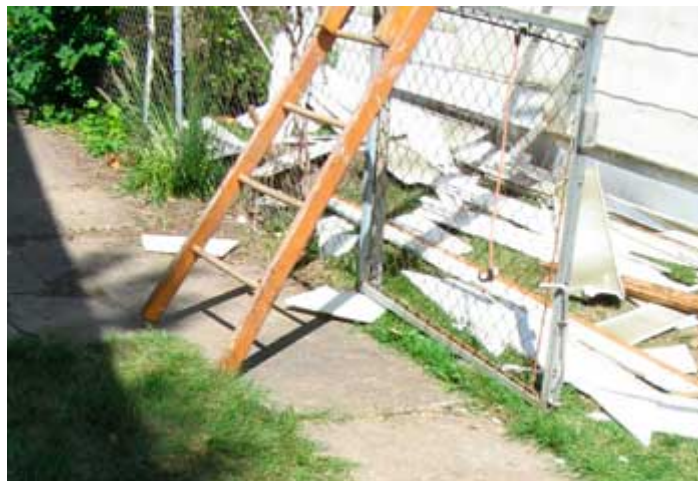
Figure 2. Ladder without safety feet on driveway against fence/gate.
