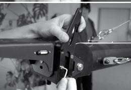
b) First of all, scroll down the tensioner pulley in the oblong hole of the central section. Now mount the tubing clamp on the upper end of the oblong hole.
