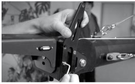
b) Fix the tubing clamp on the central section. Remove the tensioner pulley from the oblong hole first. Now mount the tubing clamp on the upper end of the oblong hole.
