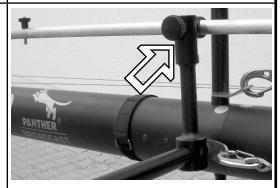
f) Use the balance rod tube with turnbuckle at the front end. Fix it on the bracket of the remote mount. Level the remote mount with turnbuckle.
