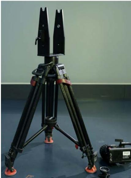
Adjust tripod to requested height and secure safely. Dismount Fluid Head (if mounted) and put central pivot section of Multiglider on top of tripod. Secure with locking knob of FluidHead.
