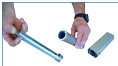
Before operation, and if required, the telescopic tubes must be degreased to ensure maximum stability.
