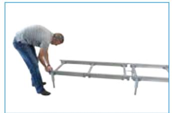
To set up the tracks please level one track first with telescopic tubes in each corner. Then connect the next track to the first one with a tie brace (1). Lift the second track and level the track with telescopic tubes at the front tube adapters. Repeat this until all tracks to be set up are levelled. At last please mount all telescopic tubes at the remaining tube adapters.
