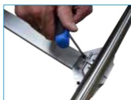
The tracks can be mounted foldable for easy transportation or fixed. To assemble the track with a fixed track gauge use a second M6 counter sunk bolt.
