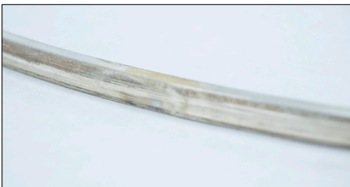
Example 2: uneven plating & wear
