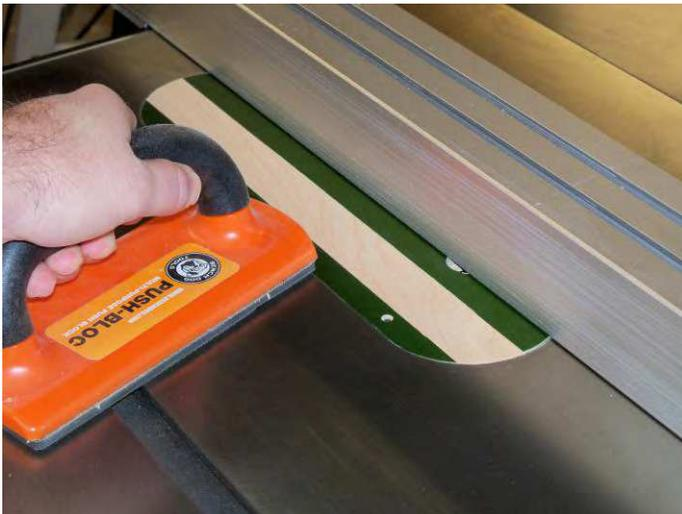
Slide in a fresh insert, set the rip fence over the throat plate (but not over the insert) turn the saw on and elevate the blade one full turn. This should cut a clearance groove in the underside of the insert, but not come out the top. Now the full 10" blade should spin freely below the insert. Make the first cut through the fresh insert with the rip fence covering the throat plate just like described above.
