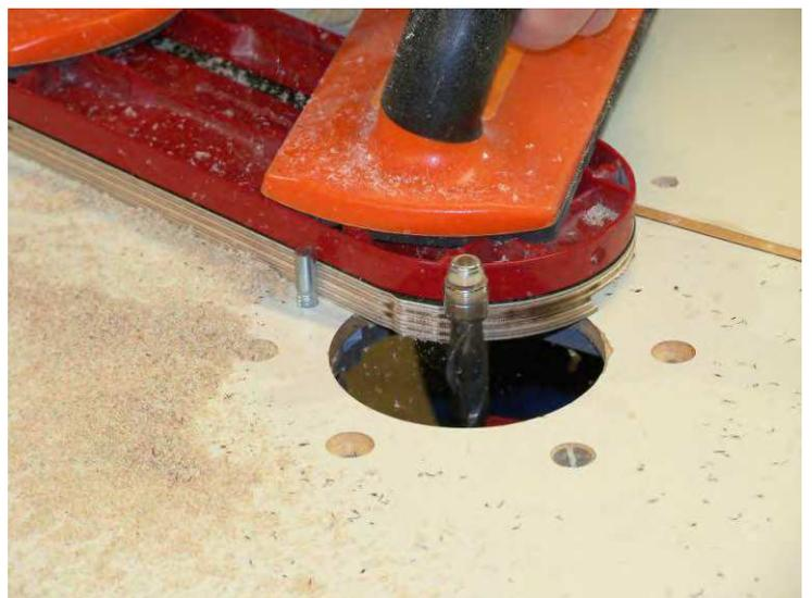
along the factory throat plate, then trim your base plate and end caps flush. The retaining pin on your factory plate will leave a tab behind, be sure to remove it when you separate the factory plate from your base.
