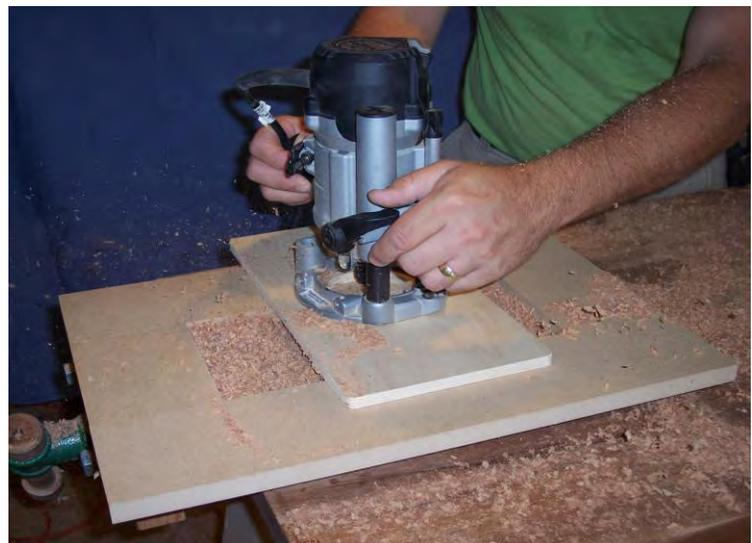
With the well milled out, a shoulder needs to be cut around the perimeter of the well for the lid panel to sit in. Simply chuck a Rabbet Bit in the router, and mill a ½ inch wide, ¼ inch deep rabbet around the edge of the well.
