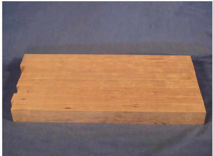
Keeping the parts as flat and square as possible during clamping will make cleaning up and milling the body much easier. Scrape any excess glue from the faces and flatten one face of the blank. This is most easily done with a jointer, but a few minutes with a sharp hand plane will do the trick too. Plane the blank to its final 1 ¼" thickness and crosscut it to 16".
