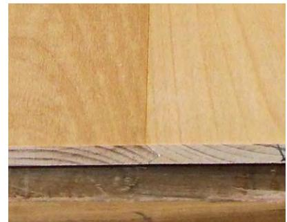
When dry, clean up the glue lines and trim the blank to fit the rabbet. The lid does not want to be too snug in the opening, room needs to be left for the natural movement of the wood. Leave about 1/16" overall. The rabbet is ¼" deep and the lid was resawn to a bit over ¼". I found that sanding it in place on the body made it easy to hold and insured that it flushed out.
