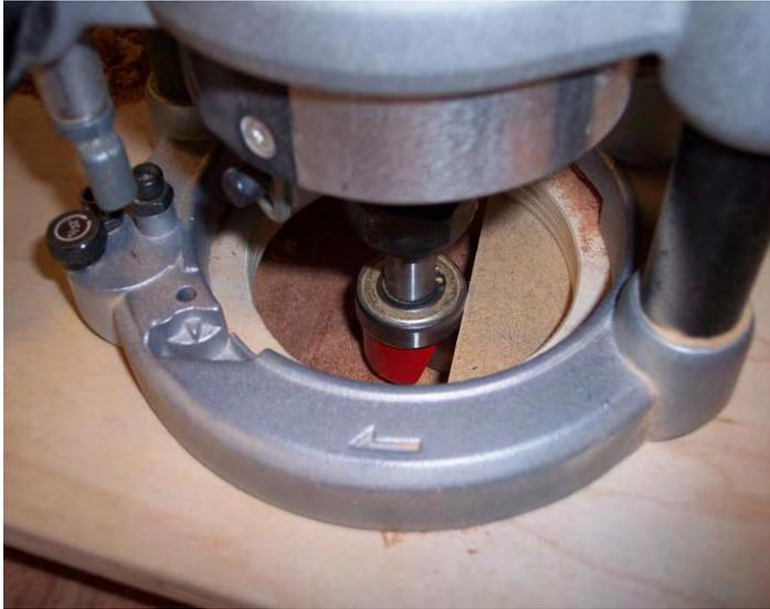
The Dish Carving Bit will leave not only a radius in the corners of the well, but also where the sides meet the bottom. A round nosed bit can do the same, but since it has no flat at the tip it does not tend to leave a clean, flat bottom in the dished area.
