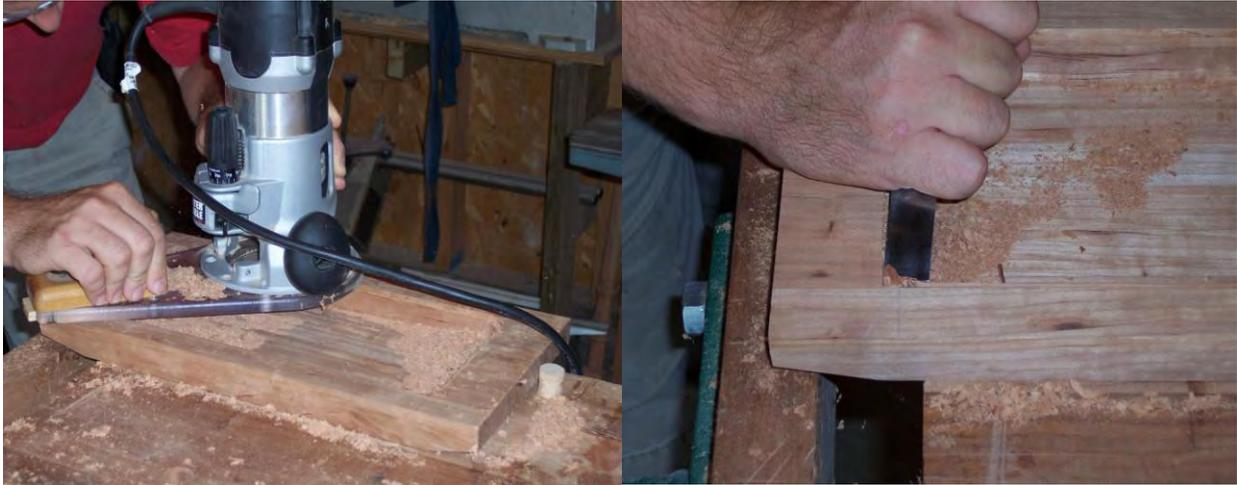
The rabbet bit will leave rounded corners that will need to be squared up. A sharp chisel and mallet will make short work of this.
