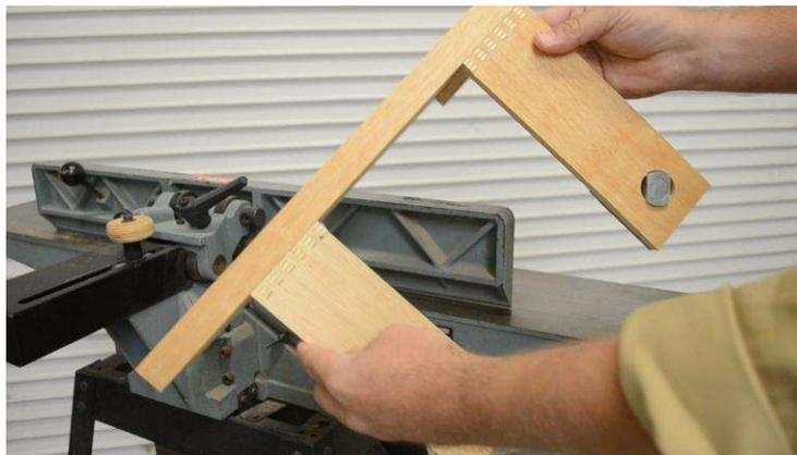
The leg assemblies need to be drilled for the magnets. We selected MagSwitch MagJig 95s which require a 1 1/4" hole. You can use rare earth magnets, but you'll need to determine hole size and placement. The
