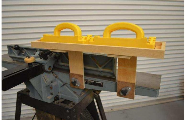
Finally, the legs are glued and nailed to the bottom of the shelf about 4" in from each end. Again, check your jointer and adjust the spacing if needed.
