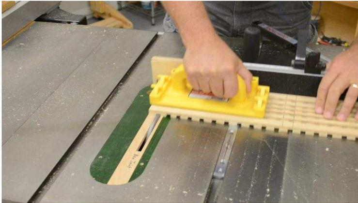
Flip the shelf over and cross cut a series of dados. The grooves and dados should overlap creating openings in the shelf for debris to fall through. This will help keep your GRR-RIP BLOCKS clean.
