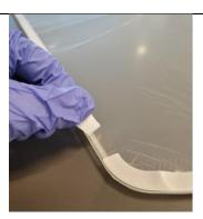
4. To position the GelMat for adhesion, it is recommended to hold the shorter edges with your fingers and place the GelMat down with its center hanging, creating a U-shape.
