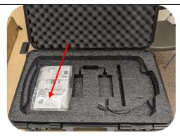
3. Fold the power cord half 3 times and use a wire tie to secure it. Then place it in the slot shown.
