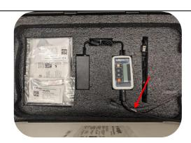
6. Gently place the Skylife unit on the foam as shown, close the lid, and secure with latches/lock.
