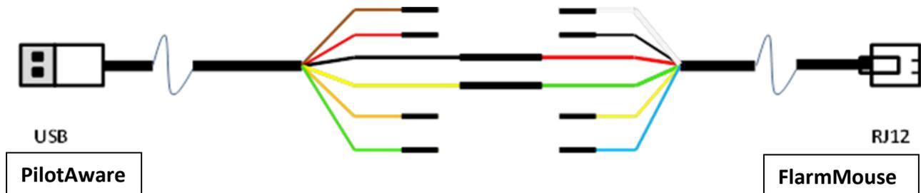
For increased security and electrical integrity, once the joints have been mechanically twisted together, the application of a very small amount of solder will permanently secure the joints, but BE CAREFUL. Applying too much heat will make the wires brittle and may also shrink the heat-shrink sleeving before you have time to move it properly into place. To minimize this risk, carefully blow the joint to cool it as soon as the solder has taken.
