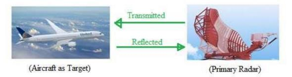
Figure-1 depicts the **primary radar** principle of operation. As shown, Primary Surveillance Radar (PSR) transmits electromagnetic signal energy towards the target aircraft. The aircraft acts as **a passive element** and reflects the EM energy back towards the primary radar antenna.
