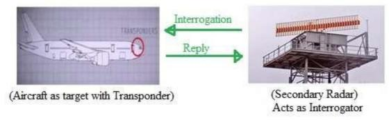
Figure-2 shows the **secondary radar** principle of operation. As shown, Secondary Surveillance Radar (SSR) transmits a signal at 1030MHz towards the target aircraft. The aircraft acts as an **active element** and its Mode-S transponder responds to this interrogation by transmitting a coded reply signal back at 1090MHz. The response contains information including its unique ICAO (Hex) Code and altitude data.
