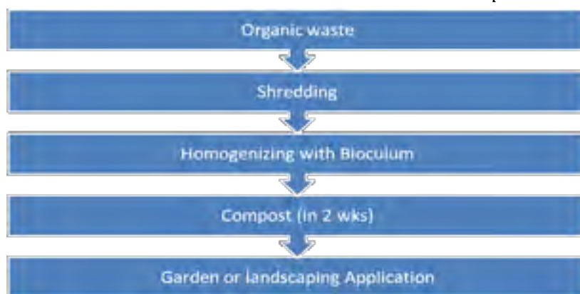
Figure 2.30 Mechanical Composting Process
