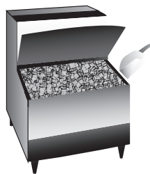
Turn off toggle switch & clean out all ice.
