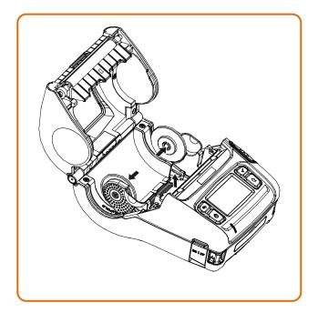
After keeping the paper guide wide as shown in the figure, hold the paper guide by lifting right guide holder as shown in the figure.
