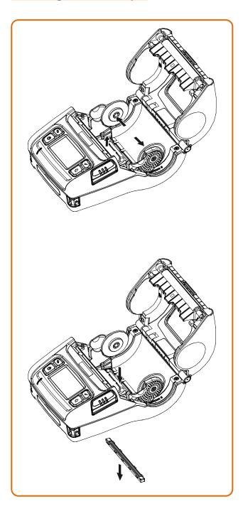
1) After keeping the paper guide wide as shown in the figure, hold the paper guide by lifting left guide holder as shown in the figure.
