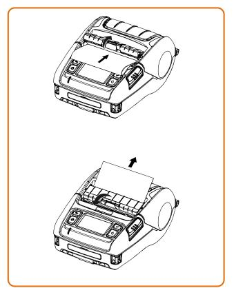
1) Insert the paper after open the peeler as shown.
