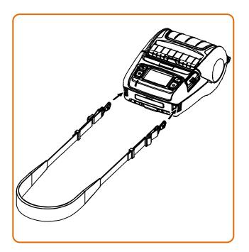
Please, insert hooks of the strap into each slot as shown in the picture.
