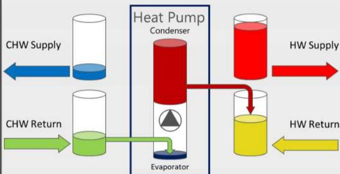
A heat pump is a thermal energy quality increaser. It collects heat from a lower temperature fluid and makes it warmer so it can flow into another warmer fluid.
