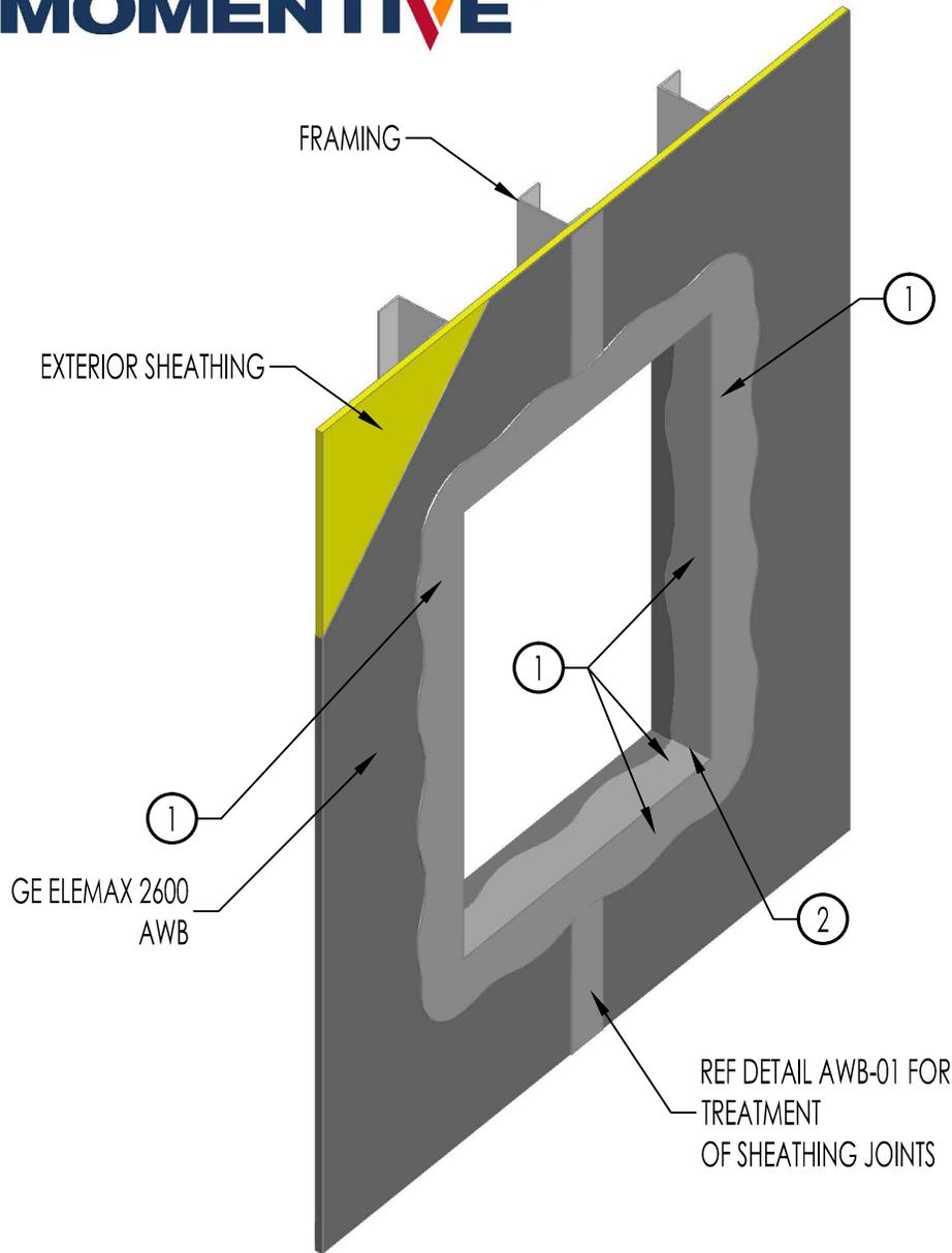
1. APPLY GE ELEMEX 5000 LIQUID FLASHING TO THE ROUGH OPENING AT A NOMINAL 20-40 MILS (508-1016 μ) THICKNESS. SPREAD/TROWEL THE GE ELEMEX 5000 LIQUID FLASHING TO A MINIMUM OF 3" (75 MM) ONTO WALL AND 3" (75 MM) INTO ROUGH OPENING. LIQUID FLASHING SHOULD BE CONTINUOUS AND SMOOTH WHILE FREE OF POCKETS, VOIDS AND/OR PINHOLES.
