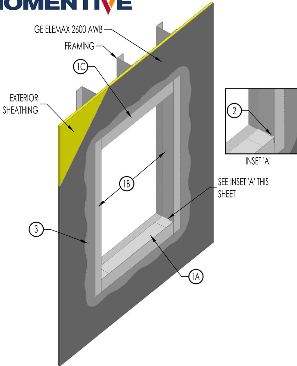
1: CUT MINIMUM 6" (152 MM) GE ELEMEX SS FLASHING SHEET TO APPROPRIATE LENGTH AND SHAPE, ADHERE IN THE FOLLOWING ORDER:
