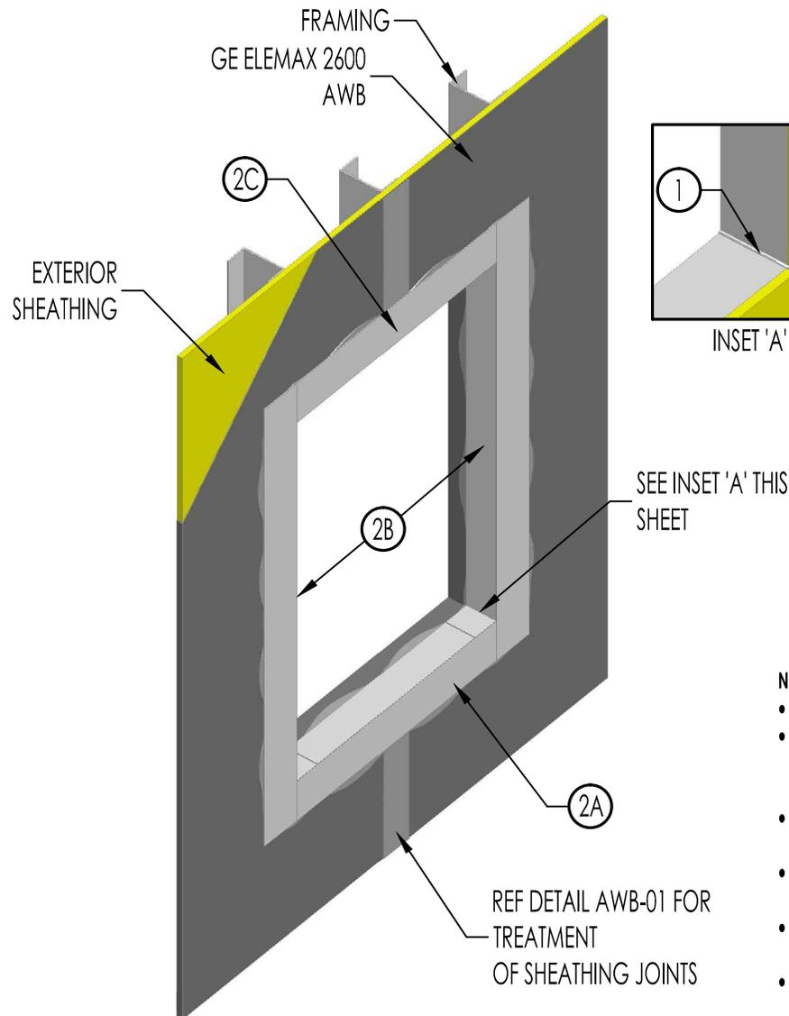
1. APPLY GE ELEMEX 5000 LIQUID FLASHING TO ALL VISIBLE GAPS, FRAMING CORNERS AND NON-FLUSH SHEATHING/FRAMING TRANSITIONS IN THE ROUGH OPENING.
