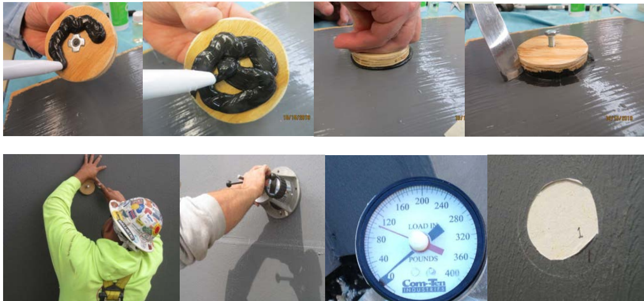
ASTM D4541 test apparatus and photos – for reference only
