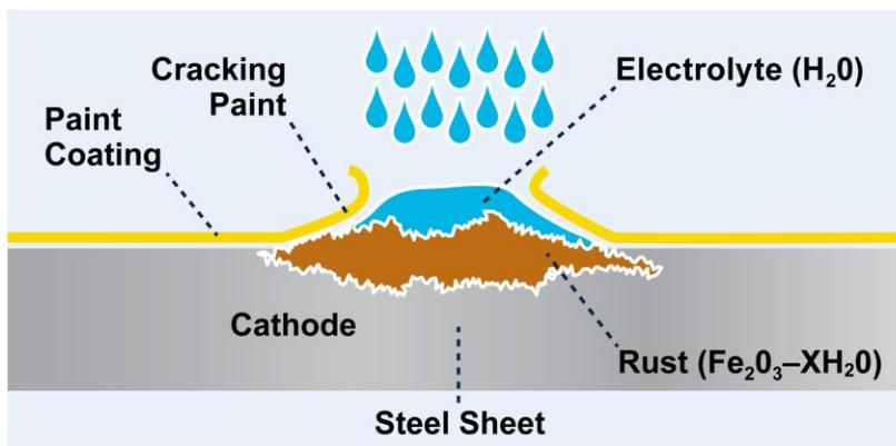
Figure 1 In order for the corrosion process to start, uncoated steel must be in contact with water and oxygen
