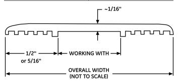
"WORKING WIDTH" is the largest joint width that can be covered.
