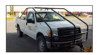
Solution: Our customer designed a robust steel cage around the cab that could be easily removed when the
