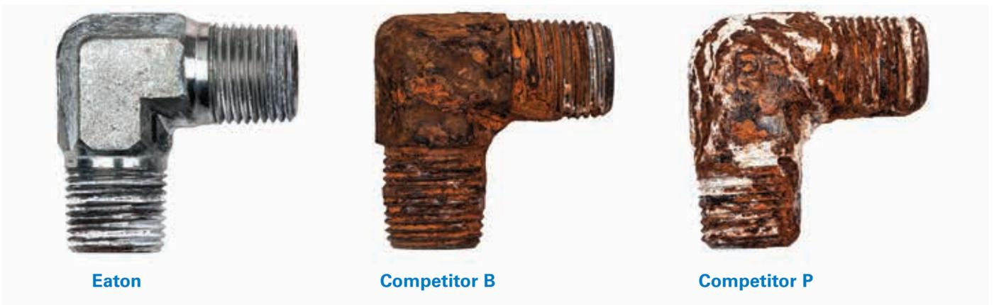
In the photos above, carbon steel fluid conveyance products protected with Eaton’s Dura-Kote plating technology resist rust longer than other carbon steel products available today.
