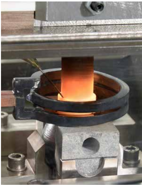
The top photo shows brazing of a heat exchanger. The bottom left photo shows high-quality banjo nipples being brazed under a controlled atmosphere in a customized EFD Induction brazing machine. Bottom right photo: Brazing of brake linings.
