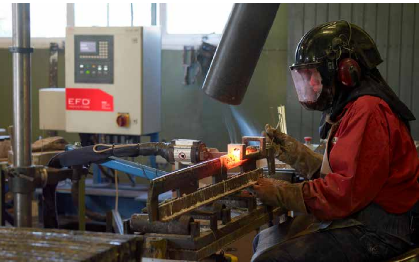
An EFD Induction Sinac heat generator in action brazing a plough share. EFD Induction products range from standard heat sources, through customized solutions to complete manufacturing processes.
