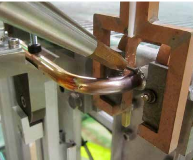
Brazing of a copper tube to an aluminium heat exchanger. Note the automatic filler material feeder.
