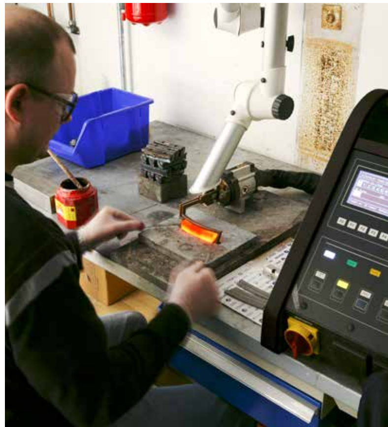
Devising brazing systems for carbide tips, blades and bits is an EFD Induction speciality. Such brazing must meet high technical standards, as the brazed joints must function in extreme working conditions.
