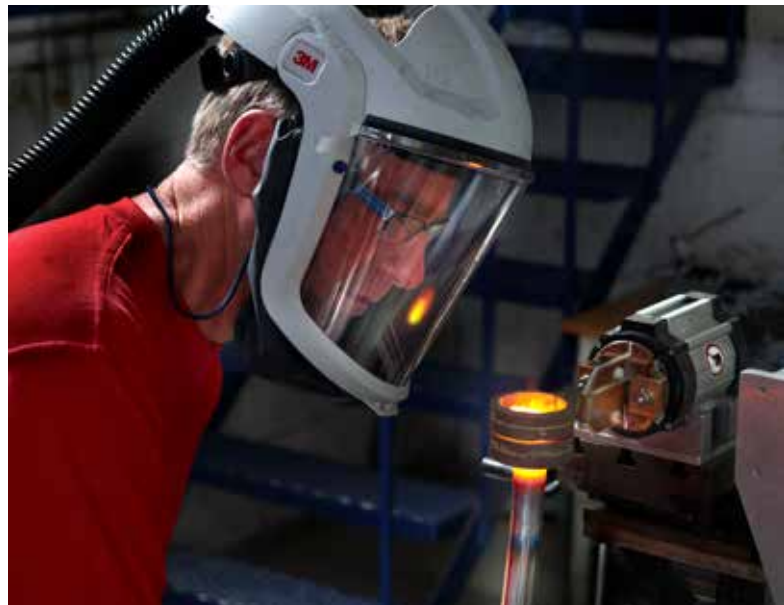
Just a few examples of EFD Induction specialist brazing solutions; brazing of a cable shoe (top), a microphone (left) and steel support bars for sofas.
