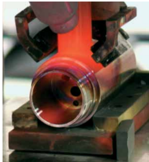
Fast, precise, controllable and easy to use. Induction is perfect for faucet brazing—whether it's tube-to-socket, tube-to-tube or thread insert brazing.
