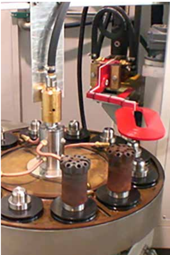
Devising brazing systems for carbide tips, blades and bits is an EFD Induction speciality. Such brazing must meet high technical standards, as the brazed joints must function in extreme working conditions.
