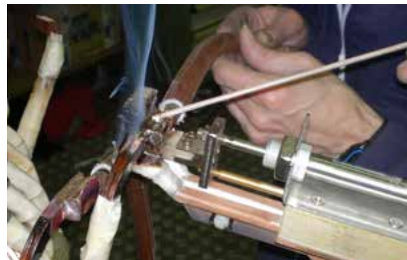
Unique design; a heat transformer with built-in clamps ensures correct positioning of parts.
