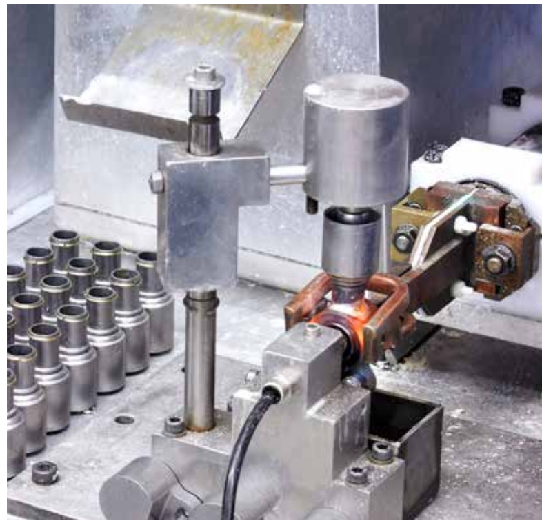
The top photo shows brazing of a heat exchanger. The bottom left photo shows high-quality banjo nipples being brazed under a controlled atmosphere in a customized EFD Induction brazing machine. Bottom right photo: Brazing of brake linings.
