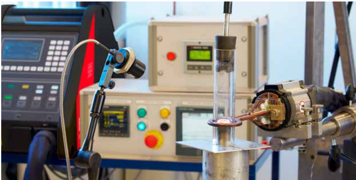
An EFD Induction Minac brazes parts for the aviation industry. Induction is ideal for brazing fan blades, blades for casings and numerous parts in fuel and hydraulic systems.
