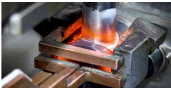
Induction heating is a perfect method for high throughput brazing of evaporator and condenser connections.
