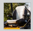
EXTRA HIGH-BACK SEAT Full mechanical suspension and additional bolstering to reduce pressure on spine and improve lumbar support.
