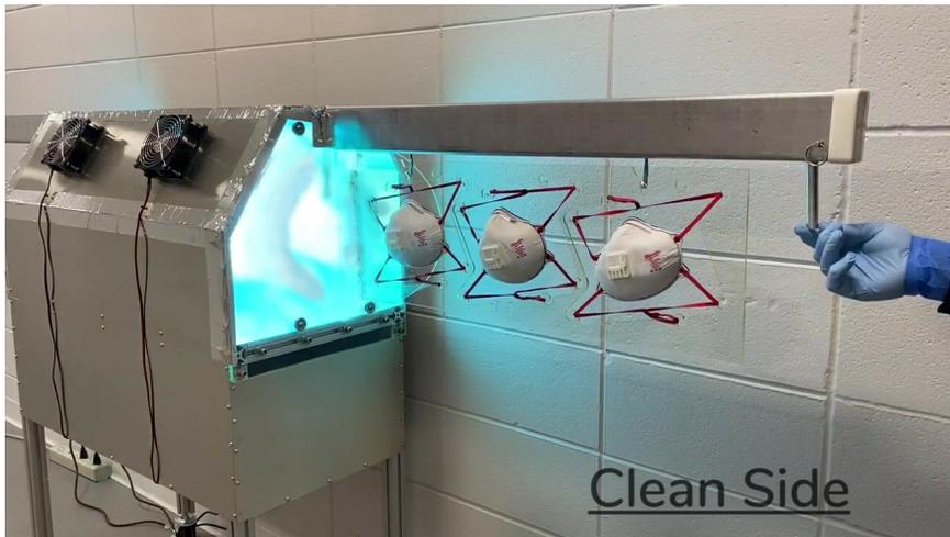
Prototype of the mask decontamination system showing UV source with proprietary bulb configuration (bottom) and rack for optimal positioning of masks within the cabinet (top).
