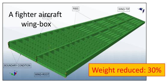
Weight reduction of 30 percent with use of DD  $[\pm 0/\pm 54]_T$  over an optimized quad in  $[0/45/0/90/-45/0/90/45]_S$
