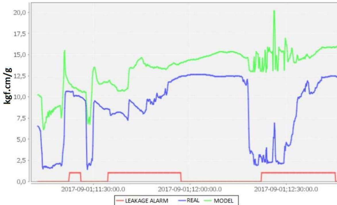
Figure 7 Real occurrences of pipeline leakage
