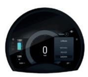
**Sherpa Mode:** the energy saving mode that saves your car's energy by limiting speed and acceleration
