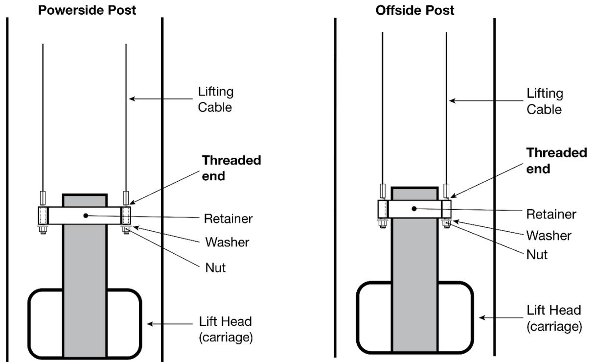
2. Place one M18 washer and M18 Nyloc nut on the threaded end.
