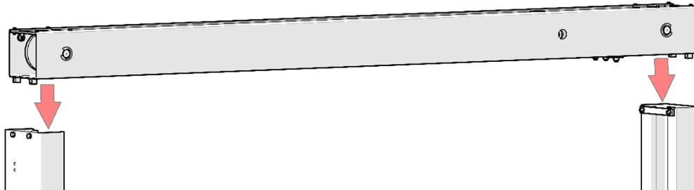
2. Align the holes on the top of the Powerside Post with the holes on the bottom of the Top Trough, then secure the Top Trough in place.
