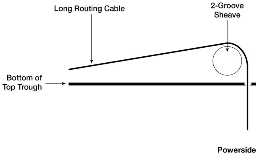
Make sure the all cables sit in the grooves and not on either edge of the sheave assembly.
