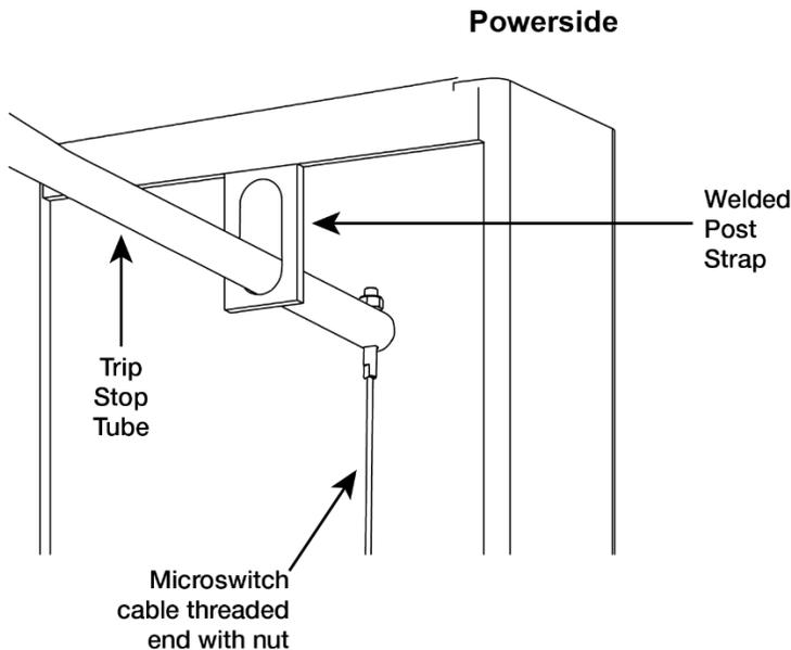
2. Route the loop end of the Microswitch Cable down the inside of the Powerside Post.
