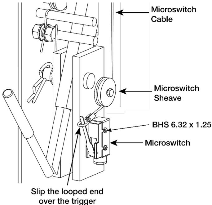
3. Put the loop end of the Microswitch Cable over the trigger on the front of the Microswitch.
