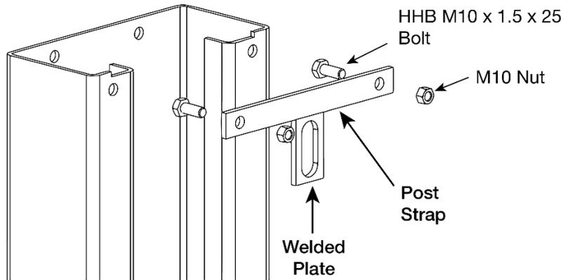
2. Bolt the other Post Strap (no welded plate) to the Offside Post.
