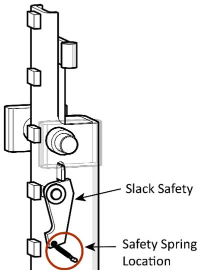
The Safety Spring should be in position, as shown in the drawing.
