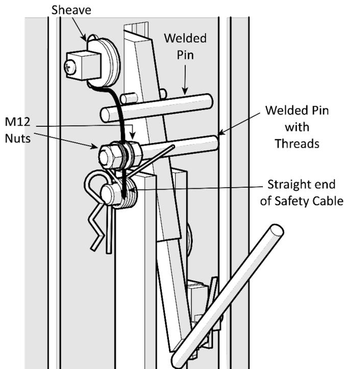
9. Operate the Safety Lock Release Handle, checking for proper operation of both Safety Assemblies.
