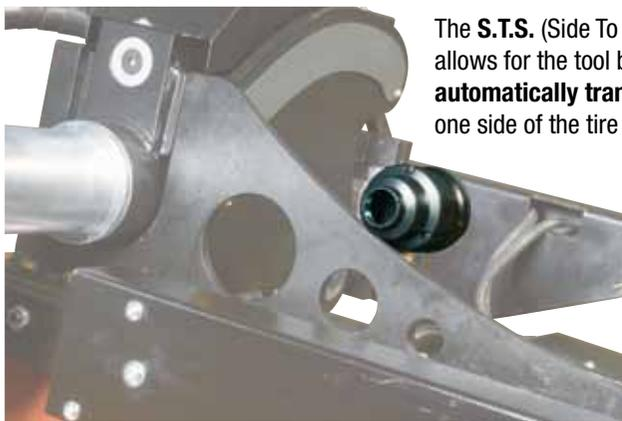
The **S.T.S. (Side To Side)** device allows for the tool block to be **automatically transferred** from one side of the tire to the other
