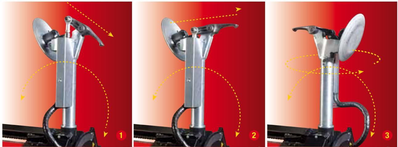
Bead breaker disc sequence of automatic movements:
