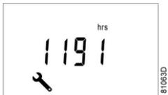
This screen shows the unit used is <hrs> (or <x1000 hrs>) and the value 1191: the compressor has run 1191 h since the previous service.
