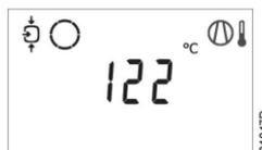
The screen shows that the temperature at the outlet of the compressor element is 122°C (251,6 °F).
