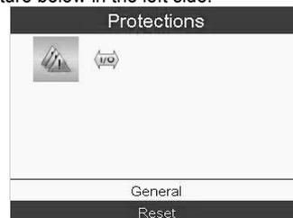
To check which is the warning, highlight the yellow triangle, using the Scroll keys. Press the Enter key and it will appear the Protections menu as in picture above in the right side. Press Enter key and then in the display will appear the list of the Protection that are active on the controller. Use Scroll key to check all the protections and the one who is causing the warning will be highlighted as in picture below:
