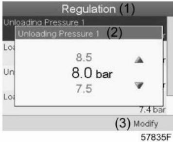
The upper and lower limit of the setting is shown in grey, the actual setting is shown in black. Use the ↑ or ↓ key of the Scroll keys to modify the settings as required and press the Enter key to accept.
