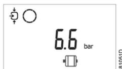
Warning: The symbol of "Motor Overload" appears both in case of an alarm in the event of converter fault or temperature switches TSHH11-12 have been tripped.
