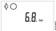
Press the scroll key (14) until the screen <d.06> appears, then press enter key (5):
