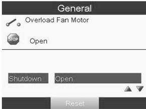
Take care that the shut-down “Overload motor” appears in case of main motor fan motor OVERLOAD or overtemperature detected by temperature switch.
