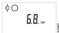
The display is showing that the compressor is running loaded (when the horizontal arrow is blinking) and the outlet pressure is 6.8bar. Consult the service dept. if <test> appears on the display.
