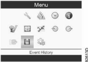
Press the Enter key. The list of last shut-down and emergency stop cases is shown.
