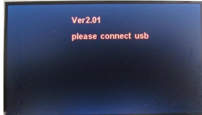
Connect the machine with PC through USB port. In PC, run USBload.exe, the PC displays the following message:
