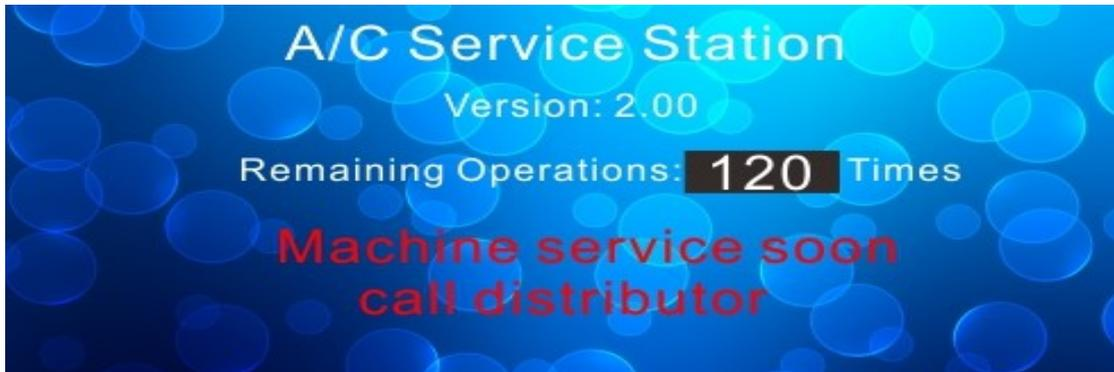
Upon 600 operations having been made, the machine will display the following message while the machine stops working. Maintenance has to be made to reset service interval time again.
