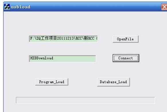
Click “Program\_load” for main program update, or click “Database\_load” for database update, the machine displays the following:
