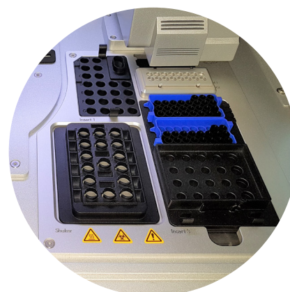
Figure 1 | PreON deck layout for TMTpro 16 plex compatible instrument
