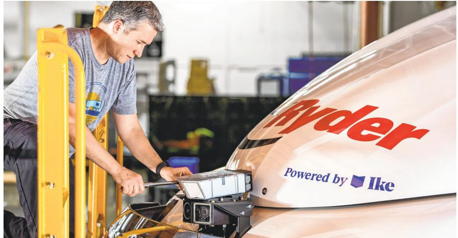
An Ike technician adjusts a sensor on the cab of a Ryder truck, part of a partnership to develop the startup's autonomous trucking technology.
