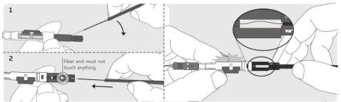
Press button on the body whilst fibre is curving.
