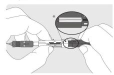
Remove the Visual Fault Locator patchcord and place the housing and fit the dust cap on the end.
