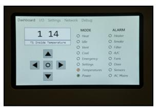
A simple user interface is provided for observing temperatures, set points and modes of operation. Secure local and remote monitoring and control can be easily duplicated using SNMP or any web browser via the internet or intranet.
