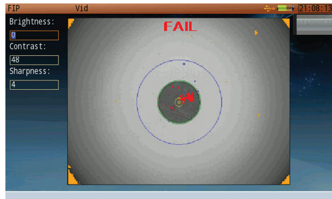
Figure 36: Fiberscope test with dirty connector.
