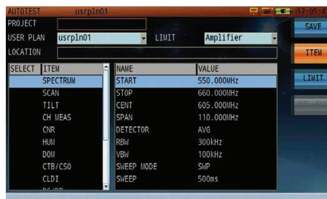
Figure 32: Define limit profiles to perform auto tests. Results will show Pass or Fail according to channel plans & limit profiles, eliminating the need for interpretation.
