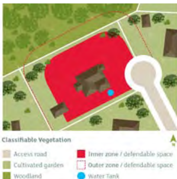
➤ Figure 14: A complex house design with poor siting prevents the required defensible space being achieved within the lot.
