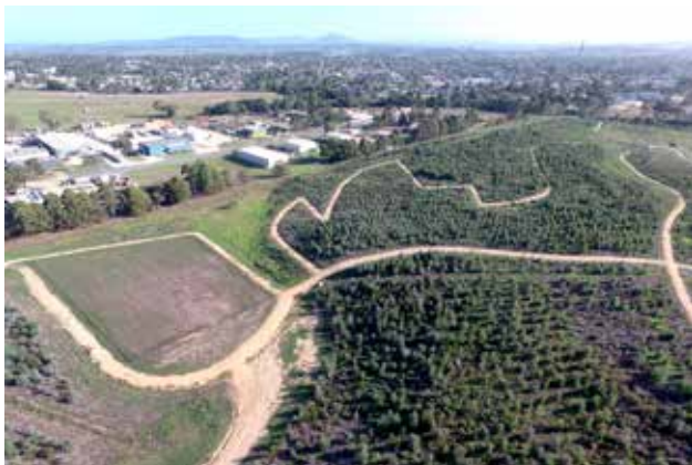
The Bosworth Road landfill in Bairnsdale was rehabilitated. The design incorporates usable public open space areas and is planted out with approximately 50,000 native trees
