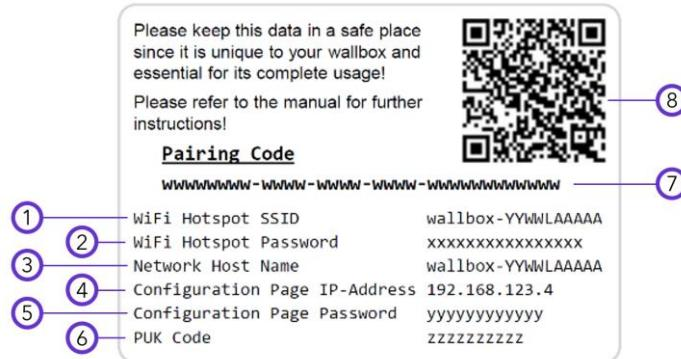
Figure 1: Descriptive illustration of the individual Configuration Sticker for each Elli Charger Connect and Elli Charger Pro
