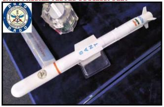
India successfully flight-tested its indigenously developed Stand-off Anti-tank (SANT) missile from Integrated Test Range (ITR) near Chandipur, off Odisha coast. The missile was test-fired from a roof-top launcher of the ground-based platform. It is an upgraded version of the anti-tank missile, Helicopter Launched Nag (HeliNa). Developed by DRDO, the missile can destroy targets 15 to 20 km away.
