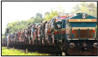
A new Roll-on-Roll off train service between Nelamangala in Bengaluru to Bale railway station in Solapur in Maharashtra was flagged off on August 31. The Ro-Ro rail, as it is called in short, is capable of transporting 42 trucks loaded with goods weighing 1,260 tonnes.
