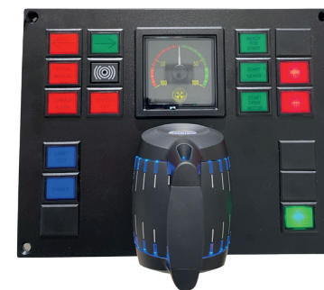
Typical new thruster panel. May be arranged to fit existing cut-out on consoles.
